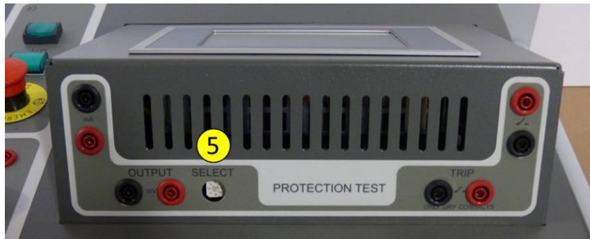
Figure 13: Interface DC Protection Test: Adjust output range.
